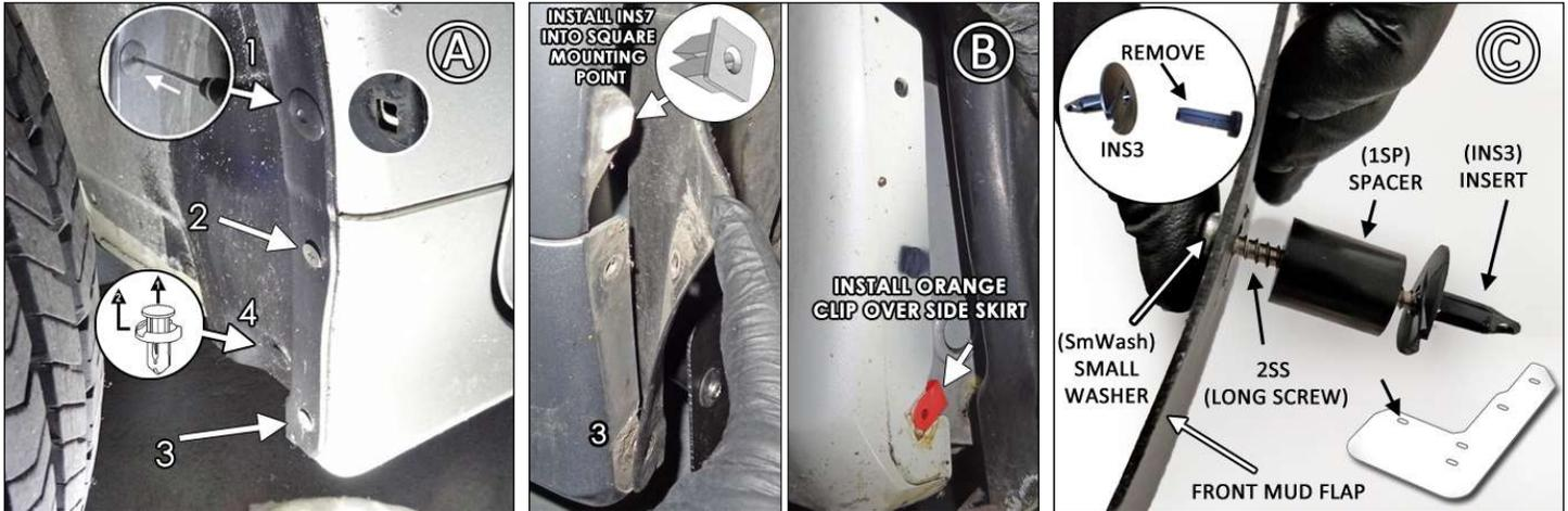
**FIGURE D** INS3 Insert assembly goes into mounting point 4. It should be firmly seated against the liner. Hold female base portion of insert securely against liner to prevent it from spinning. Continue threading the Long Screw (2SS), keeping the Insert seated against liner during this process. Tighten until washer is *almost* seated against the flap. Do not fully tighten so you can adjust later.
